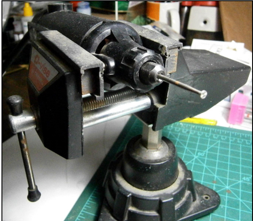
Dremel with shaping bit used to rabbet wing root
