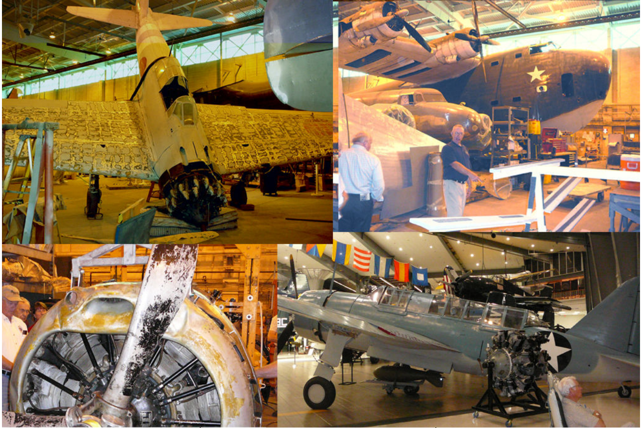
Photos from Ken Hornby's trip; Clockwise, from upper left: a real Japanese Zero under restoration; a PB2Y Coronado and other goodies; a SB2A Buccaneer; and the engine from a Brewster Model 339 (export F2A Buffalo)
